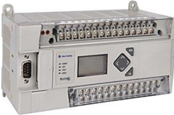
Figure 2 AB MicroLogix 1400 PLC
